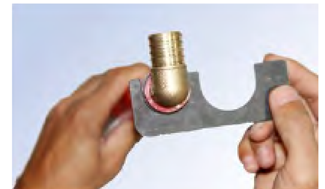
Step 5: Checking Use the GO-NO-GO gauge to check whether the pressing is completed. If the crimp ring slides into the "GO" slot, but stops at the shoulder in the "GO" slot, then the pressing is acceptable.
