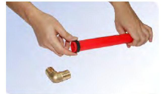
Step 2: Sleeving Choose the right size fitting according to the pipe. Put the copper crimp ring over the pipe at the right position.
