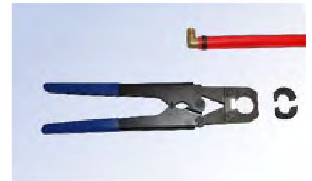
Step 3: Selecting the jaw Choose the right size of fitting and jaw of the crimping tool.
