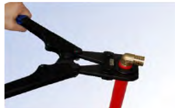
Step 4: Pressing Open the crimping tool and put the fitting into the jaw. Press the jaw until it closes completely. While pressing, make sure the crimping jaw is vertical to the pipe, the pressing contact must be free of impurity.
